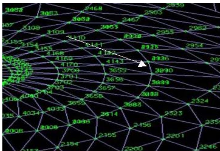
Fig (7): Verification of the final mesh for the interface of plate volumes and screw volumes. The white arrow is pointing towards the boundary of V1 and V2
