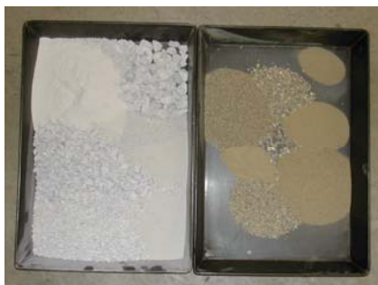
a. Manufactured and natural aggregates prepared in lab
