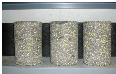
b. Asphalt mixture cores prepared in Michigan Tech
