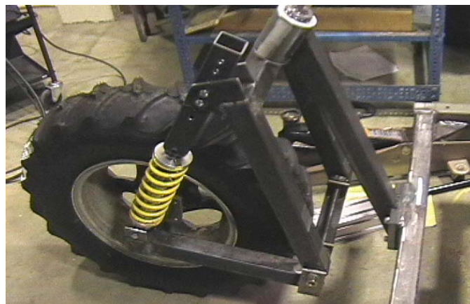
Figure 2 Photo of the constructed front end assembly of the BUV show during assembly and testing.
