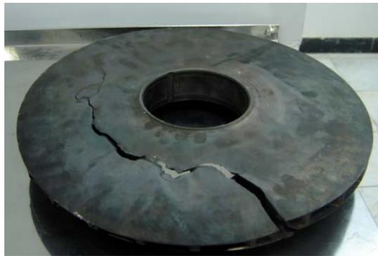
Figure 2: Fracture on Disc
