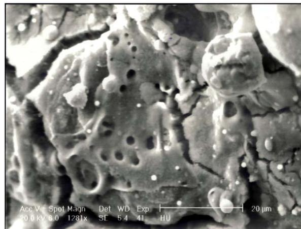
Figure 10: Detachment of Grains Due to Creep Mechanisms
