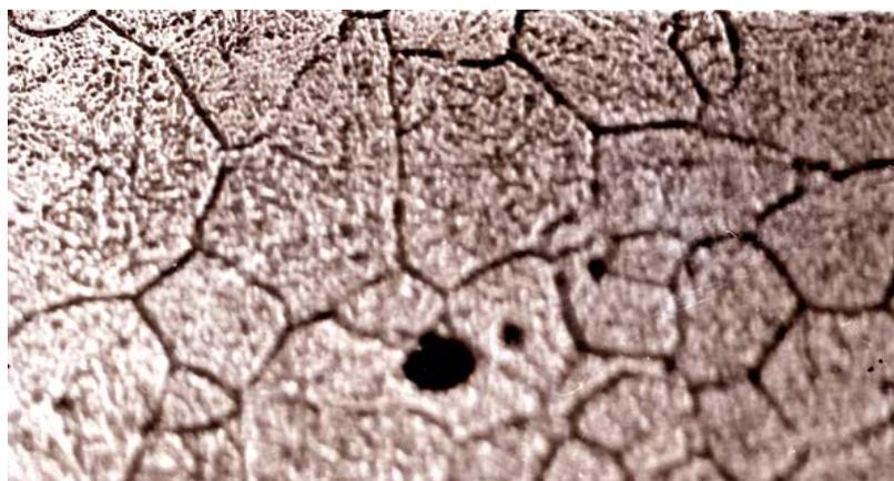
Figure 5: Macrocracks Have Formed on Grain Boundaries (200×)
