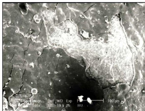
Figure 7: Fatigue Cracks on Cover Coating
