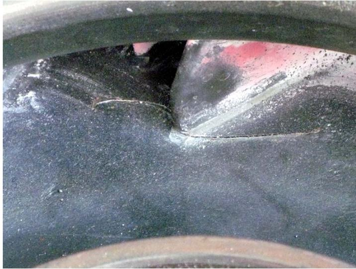
Figure 18: Crack at the Junction of Blade and Disc
