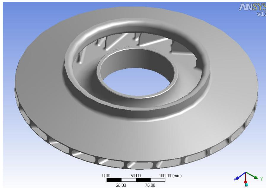
Figure 11: Mechanical Model of the Impeller
