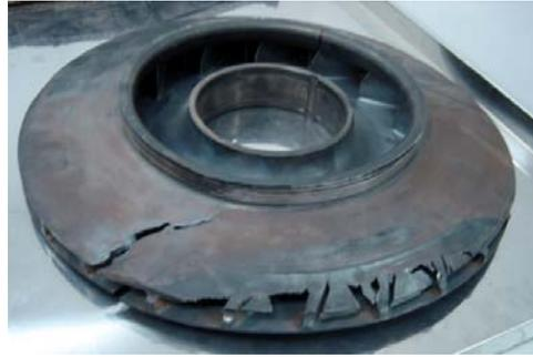
Figure 1: Fracture on Cover
