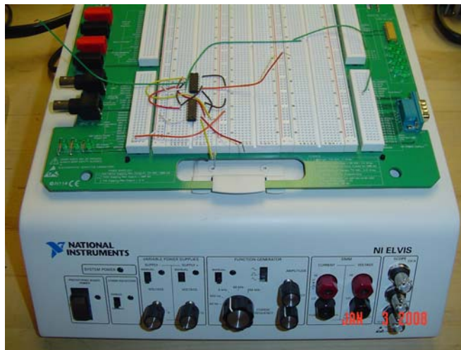
Figure 3: Prototype Control Circuit Built on a NI ELVIS Experimenter [23]
