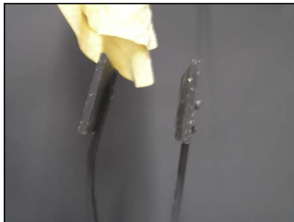
Figure 5: The fixed gripper with material edge waiting to be gripped
