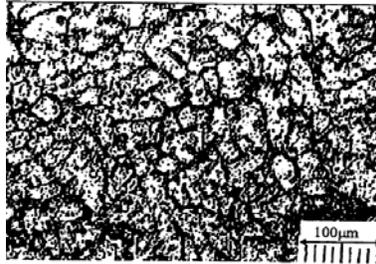
Figure 4: Size of dendrite arms for A356 casting specimens
