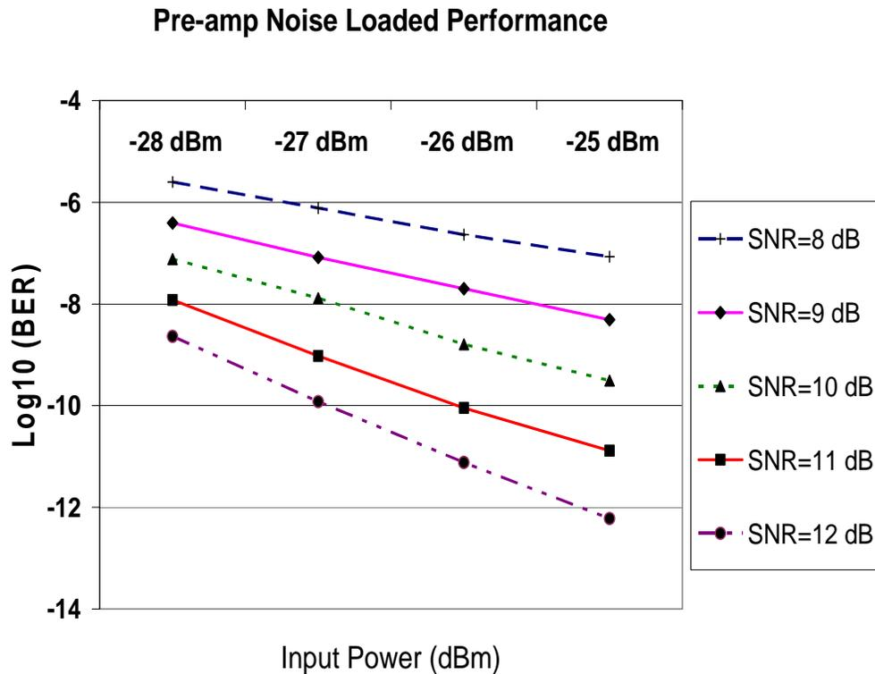
Figure 3: Optical receiver performance at different input powers and different input signal to noise ratios
