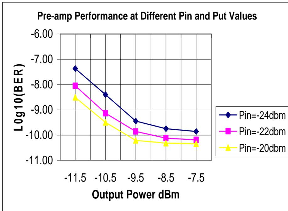
Figure 2: Optical receiver performance change at different input and output power levels
