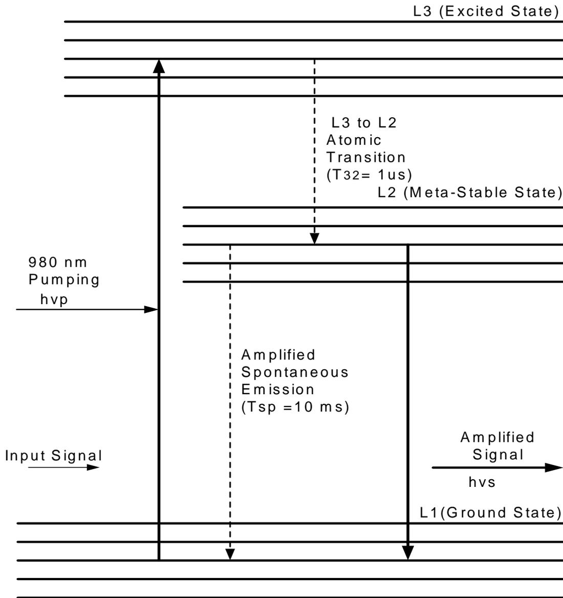
Figure1: 980 nm pumping in Erbium atomic structure
