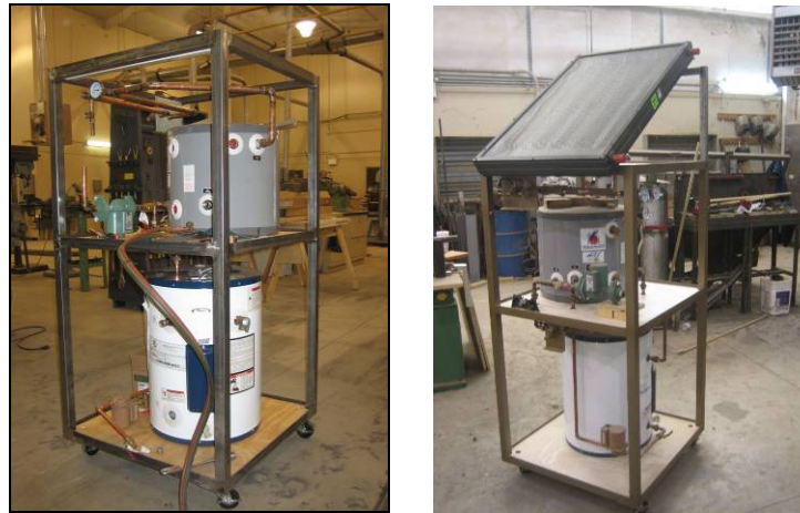
Figure 3: Passive solar water heating system
