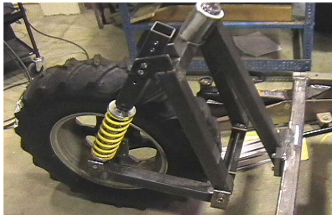
Figure 2 Photo of the constructed front end assembly of the BUV shown during assembly and testing.
