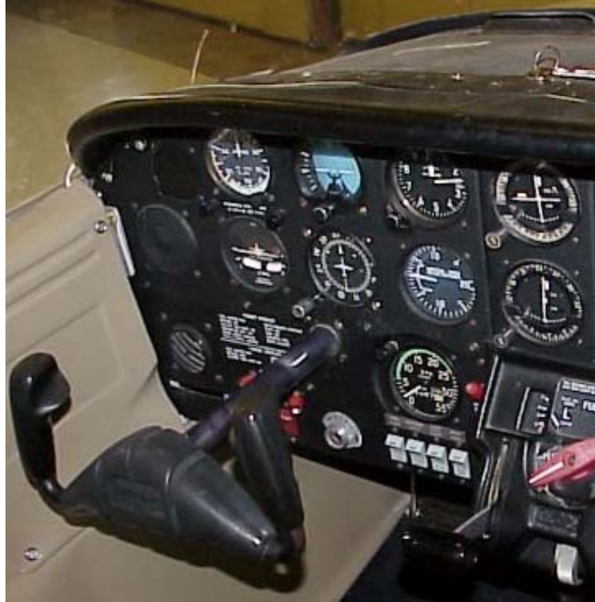
Figure 2: Cockpit of Piper Tomahawk airplane with mechanical gauges
