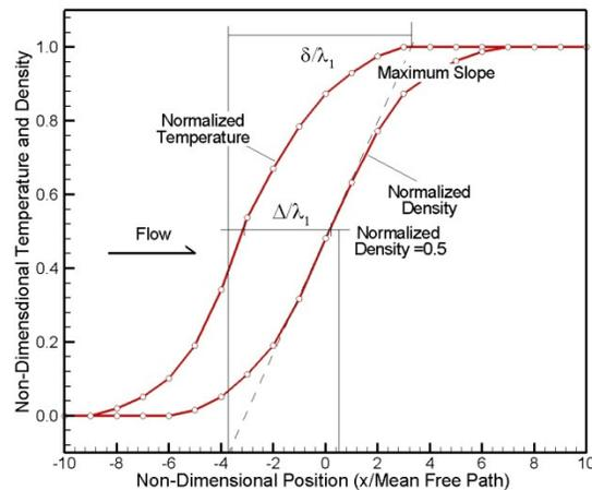
Figure 1. Schematic drawing of shockwave structure in neutral gas
