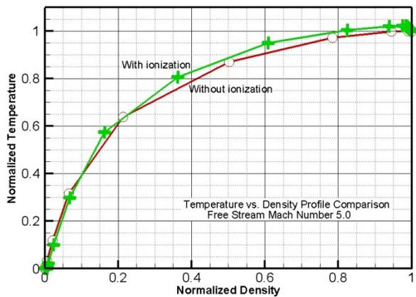
**Figure 5. Comparison of the normalized temperature-density shift between weakly ionized gas and neutral gas. Free-stream Mach number is 5, ionization fraction is 0.75 parts per million**
