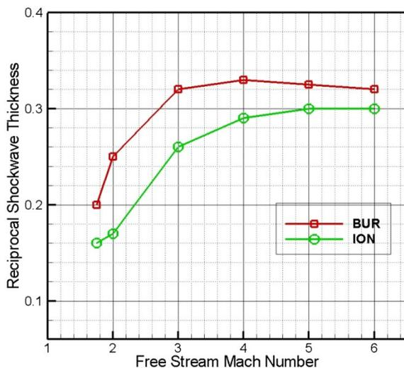
**Figure 6. Comparison of reciprocal shockwave thickness ( $\lambda_1/\delta_s$ ) between ionized argon and neutral argon gas. The ionization fraction is 0.75 parts per million**
