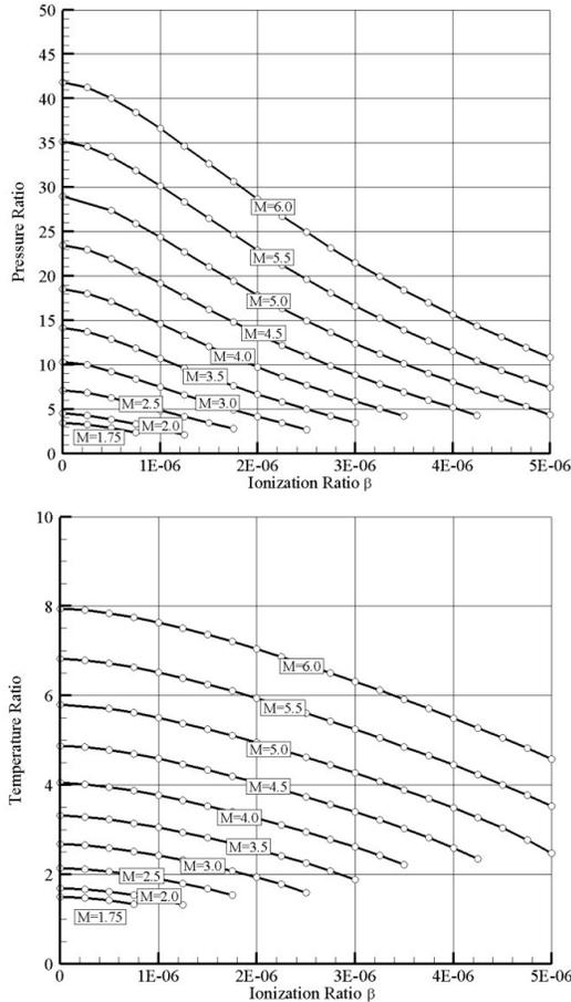
**Figure 3. Computed pressure and temperature ratios across normal shock for free-stream Mach numbers ( $M=1.75-6.0$ ) and ionization ratio  $\beta$**
