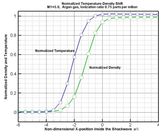
**Figure 4. Non-dimensional temperature-density profile for  $M_1=5.0$ . argon gas, ionization fraction is 0.75 parts per million**
