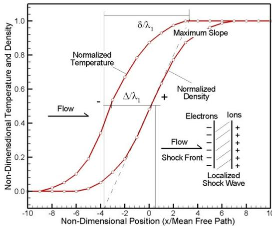
**Figure 2. Schematic shockwave structure in weakly ionized gas. Electrostatic body force exists**
