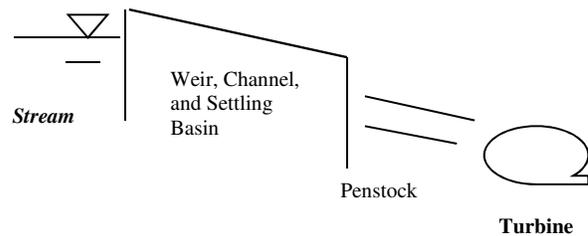
**Figure 2. Diagram of Hydroelectric Plant**
