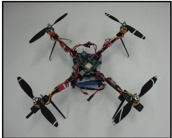
Figure 2. Quadrotor with Onboard Control
