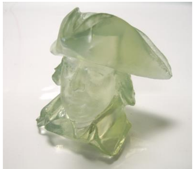
Figure 5. SLA Part Made with DSM-SOMOS Watershed 11120
