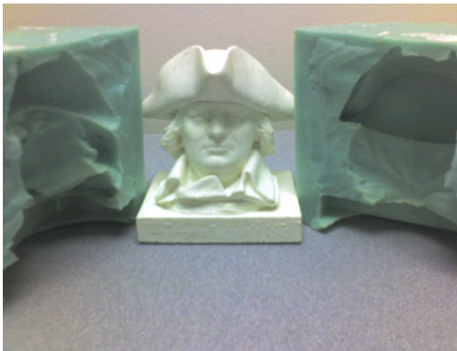
Figure 7. A Polyurethane Replica and Its Silicon Rubber Mold Halves
