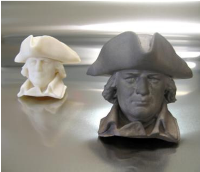
Figure 6. ABS and S4/Bronze Reproductions Made with FDM (left) and ProMetal 3D Printing (right) Technologies
