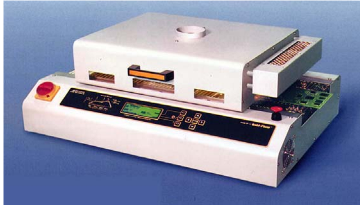
Figure 4 Reflow oven similar to the one where the experiments were conducted.
