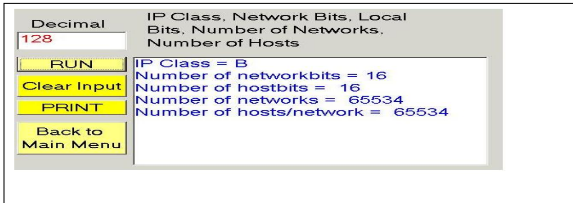
Figure 3. IP Class, Network and Host Information without Subnet
