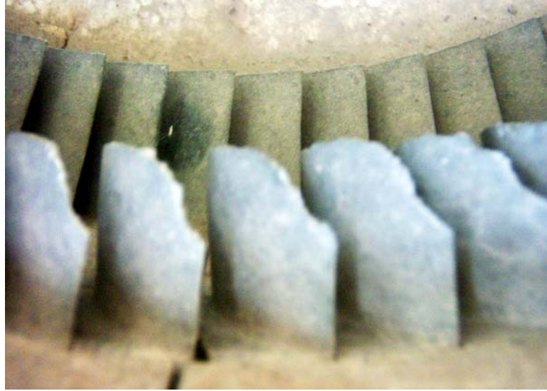
Figure 2: Failed Stator Blades
