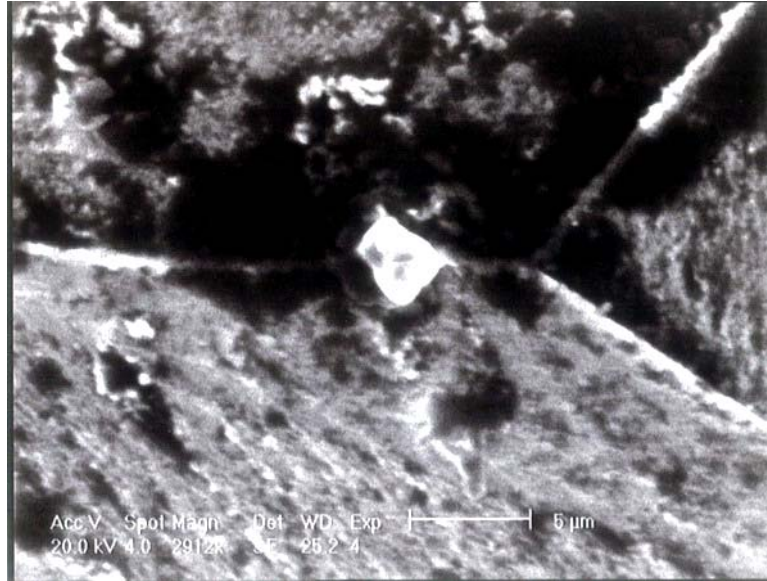
Figure 7: Dispersed Particles of Carbides Precipitates
