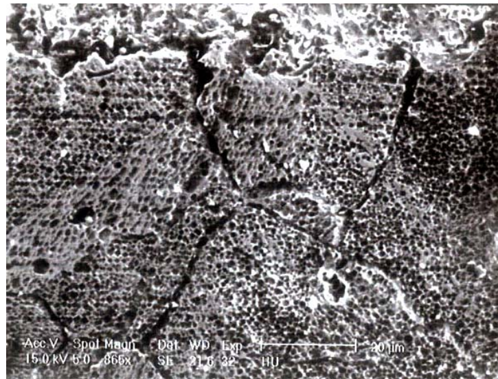
Figure 12: Several Macrocracks on Grain Boundaries Due to Creep Mechanism
