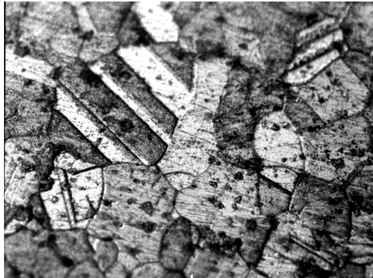
Figure 13: Annealing Twins Taken by Optical Microscopy (200×)
