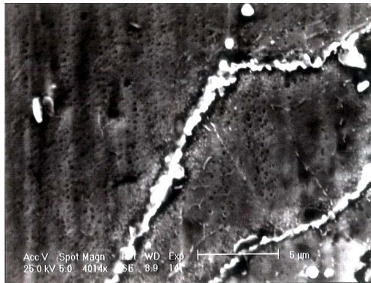
Figure 6: Continuous Films of Carbides Precipitates
