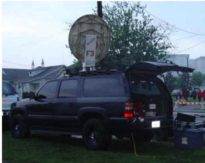
Figure 2: MITOC Satellite Dish Erected
