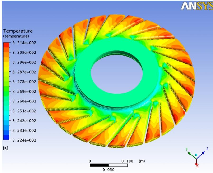
Figure 14: Flow Temperature Contour
