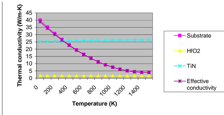
Figure 4: Effective conductivity for TiN coated tool
