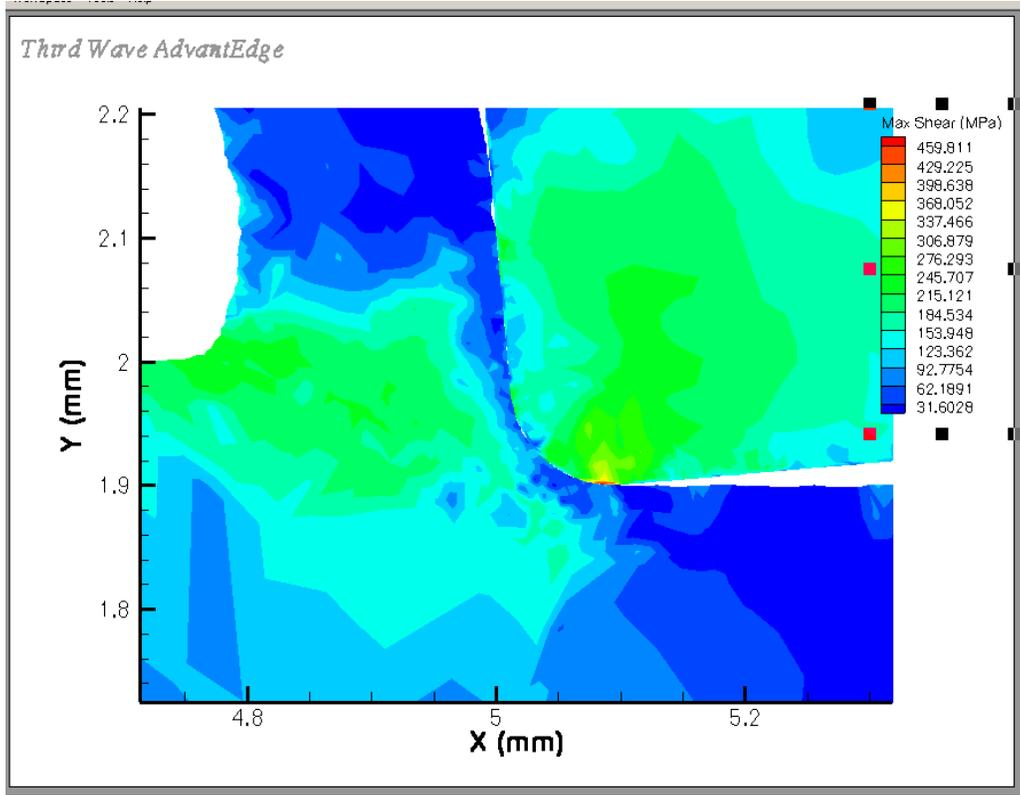
Figure 12: Shear stress distribution at  $V = 16$  m/s
