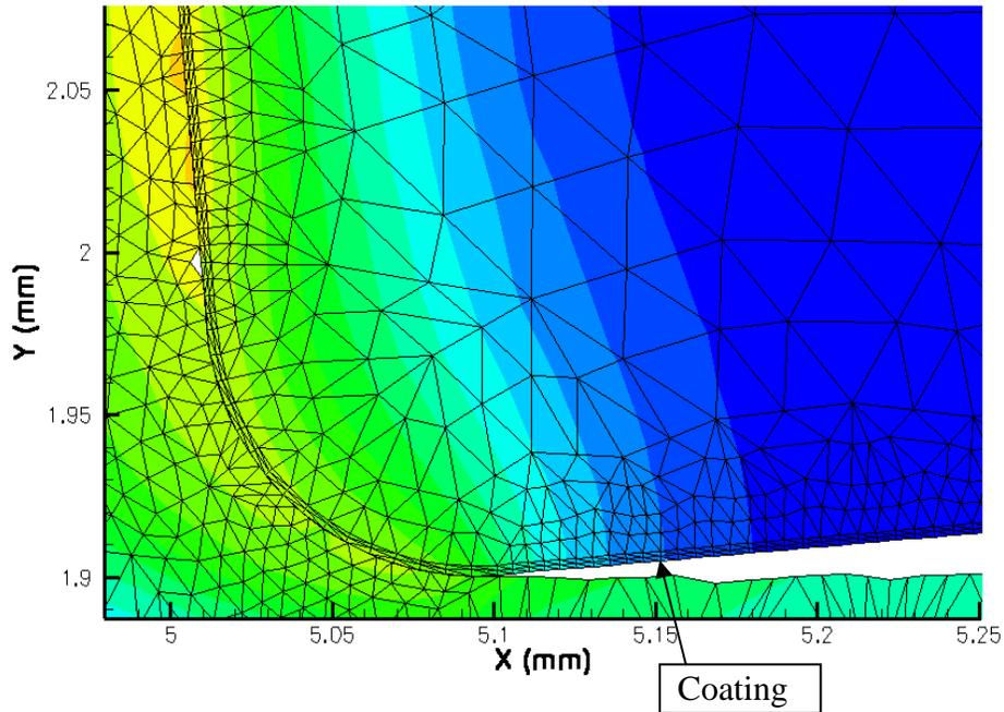
Figure 6: Tool substrate and composite coating mesh
