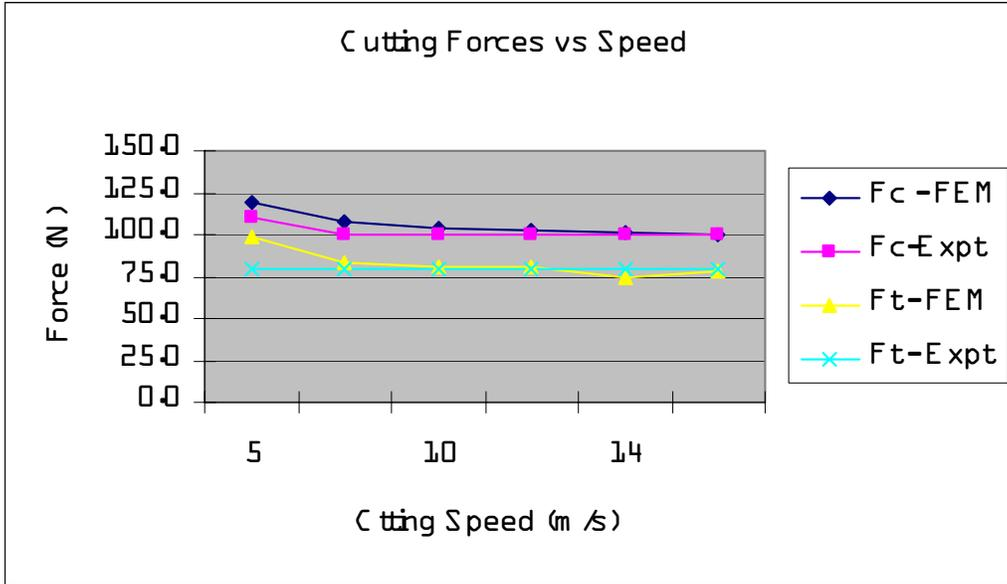
Figure 7: Comparison of simulation and experiment – cutting forces vs. cutting speed
