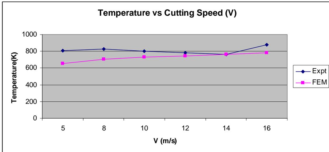
Figure 10: Peak tool temperature vs. cutting speed
