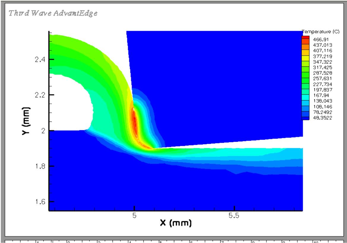
Figure 11: Temperature distribution at  $V = 16$  m/s
