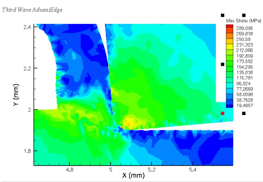
Figure 13: Shear stress distribution at  $V = 8$  m/s
