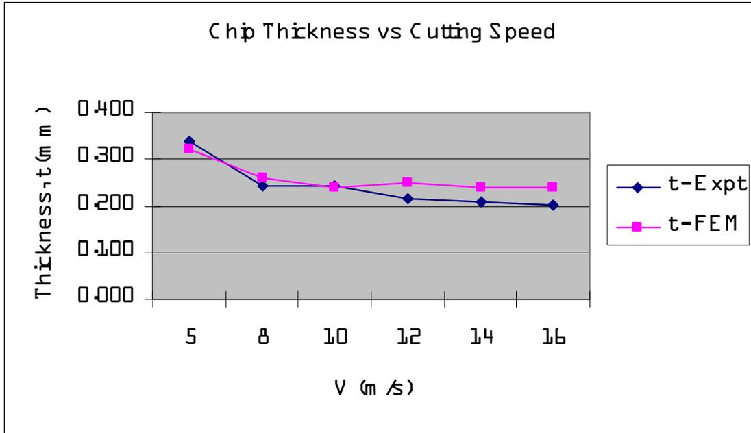
Figure 9: Chip thickness vs. cutting speed
