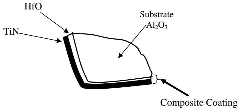
Figure 5: Composite model of the multiple coatings
