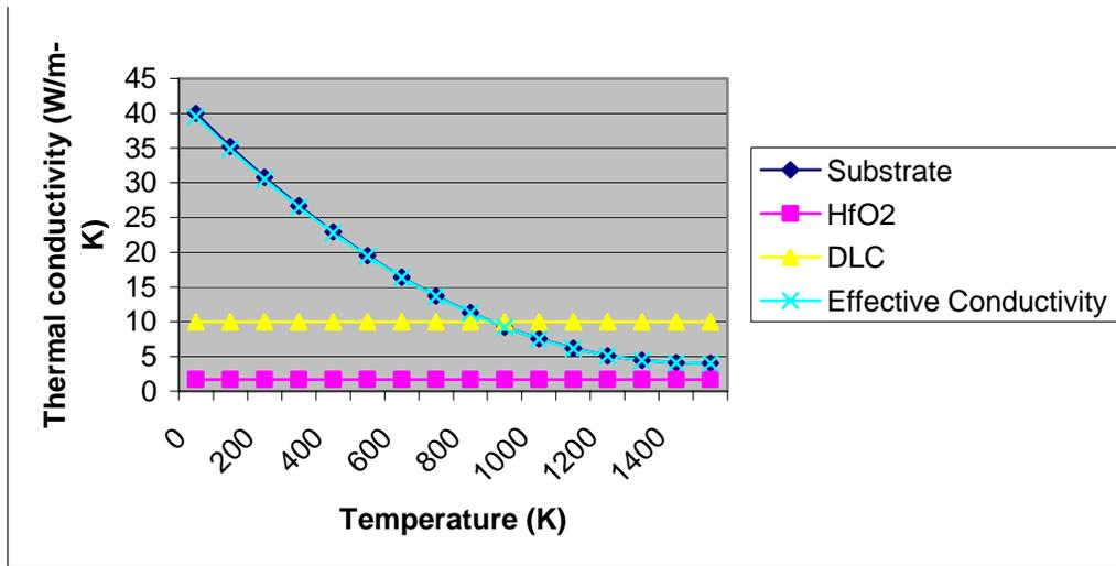
Figure 3: Effective conductivity for DLC coated tool
