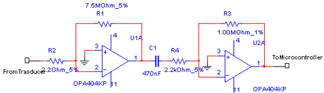
Figure 2: Custom-built Amplifiers from OPA404KP-ND for Mobile Station
