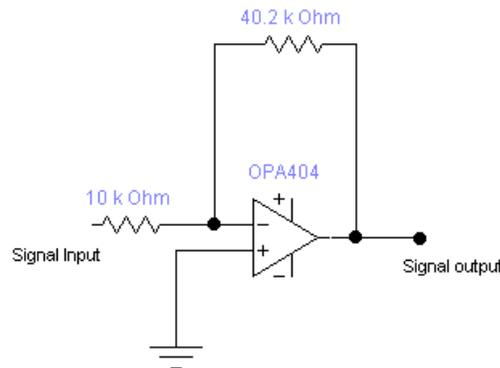
Figure 1: Custom-built Amplifiers from OPA404KP-ND for Base Station
