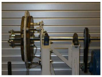
Figure 11. Laboratory setup for wind generator experiments
