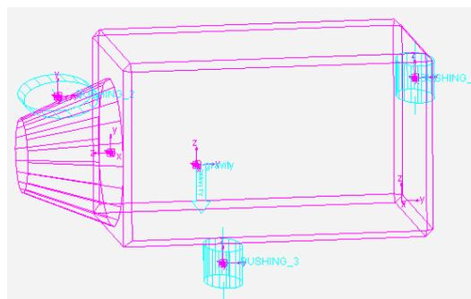
Figure 2: Powertrain dynamics model
