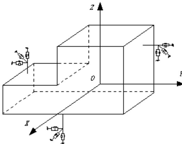
Figure 1: The mechanical model of powertrain mounting system
