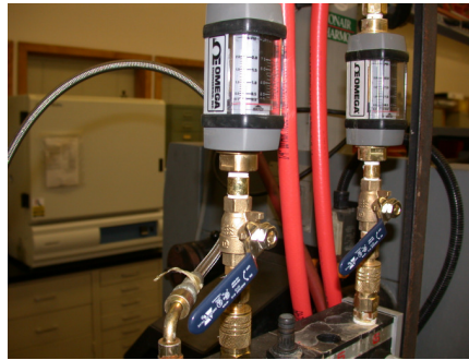
Figure 2b. Omega flow meters & ball valves.
