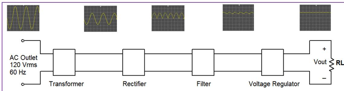
Figure 3. DC Power Supply Block Diagram
