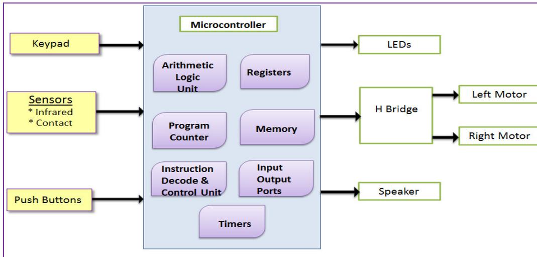
Figure 4 Typical Robotic System Block Diagram
