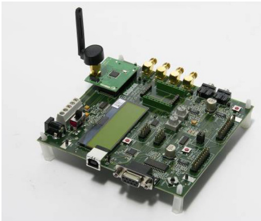
Figure 4. TI CC2430EM Module on the SmartRF Development Board
