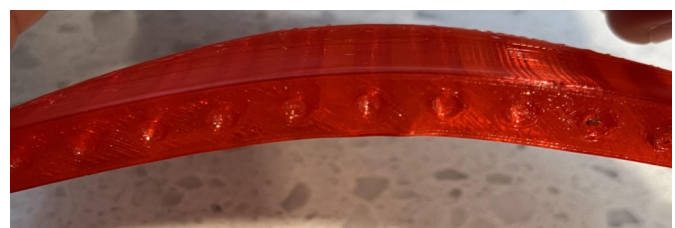
Figure 19. Demonstration of the fin deforming during the bending test within 25% of the TPU fins.
