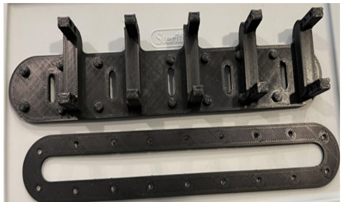
Figure 3. Additively manufactured cam system to hold servo motors.
