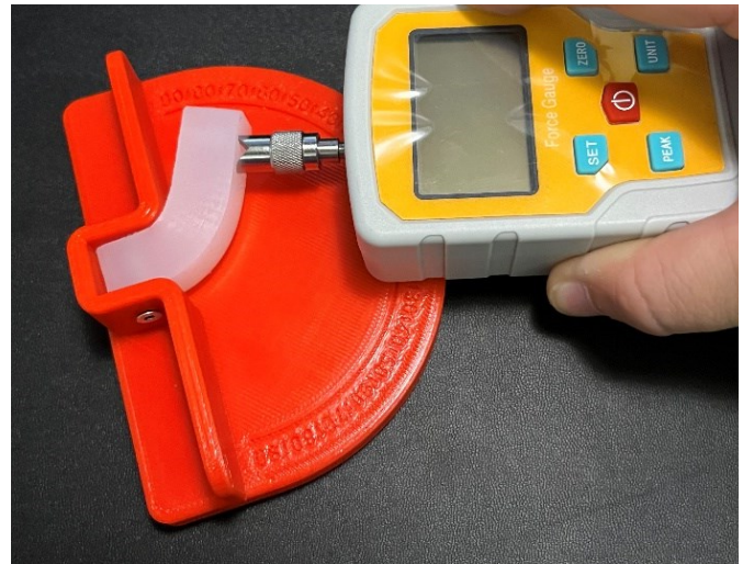
Figure 10. Force gauge position against material extrusions to accurately measure deflection.
