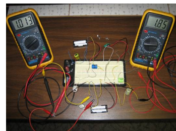
Figure 8. Battery discharging process
