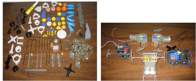
Figure 3a. Gear box components Figure 3b. Assembled gear boxes
