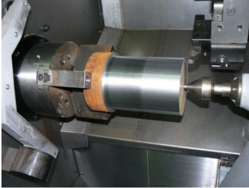
Figure 5. Workpiece after One Turning Path
