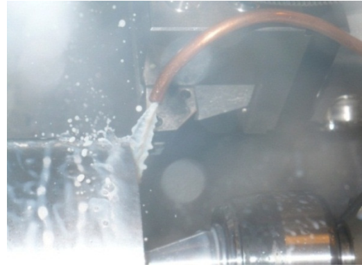
Figure 6. Cutting Fluid Applied to Insert and Workpiece
