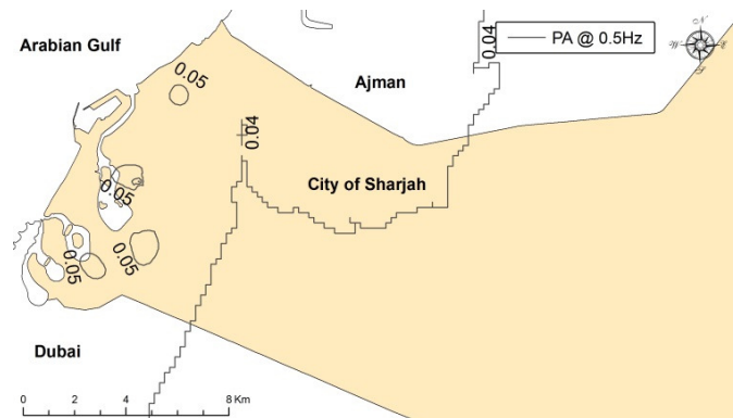
Figure 6. Spectral Acceleration Map of the City of Sharjah at 0.5 Hz
