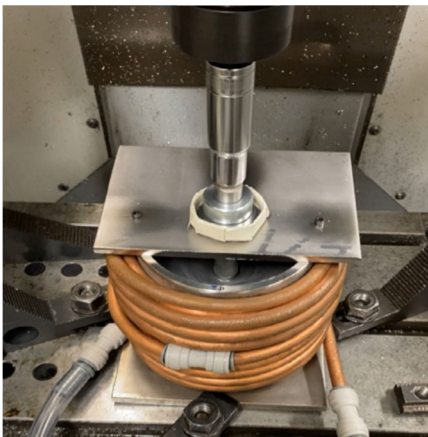
c) The completed unit with the lead opened and connected to the spindle of CNC mill.
